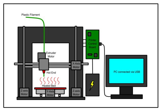
Fig. 4 Experimental Set up of 3D Printer
