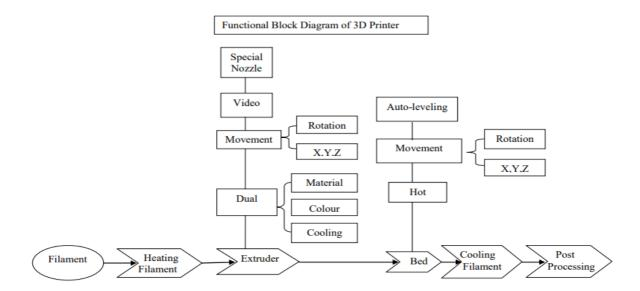
Fig. 3.1.1 Functional block diagram of 3D Printer
