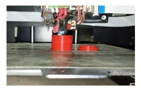
Fig 5.3.3 Actual image of Capacitor printing process
