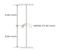
Fig. 7.1.2 Chrome platted Hardened shaft
